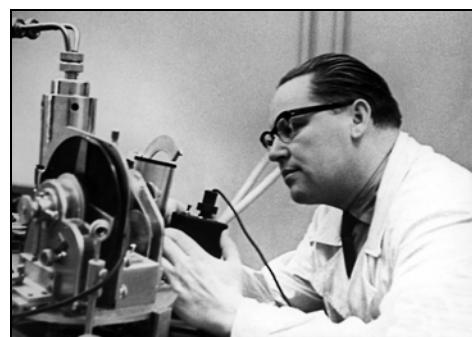
J. Bleidelis sets up the camera to photograph the reciprocal lattice of crystals, 1965
